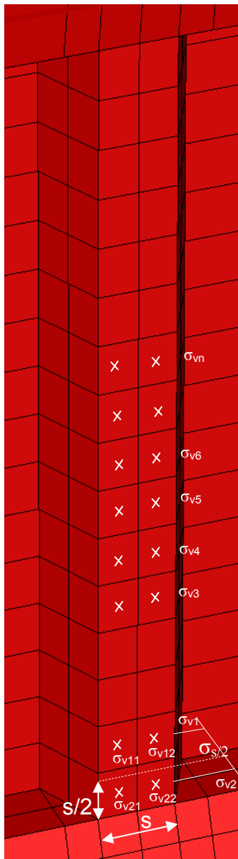
Figure PR2 Averaging and Linear Interpolation of Element Stresses for Flange Panel Buckling of Vertically Corrugated Bulkhead
