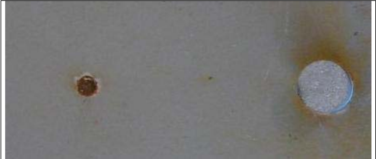
Figure C-2 Disbonding from artificial holiday, bottom wave tank panel (example picture not connected to example results in this model report).
