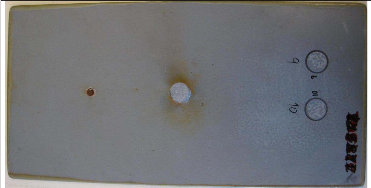
Figure C-1 Disbonding from artificial holiday, bottom wave tank panel (example picture not connected to example results in this model report).
