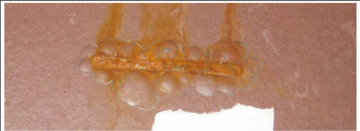
Figure C-3 Scribe area of top wave tank panel before removing of loose coating (example picture not connected to example results in this model report).
