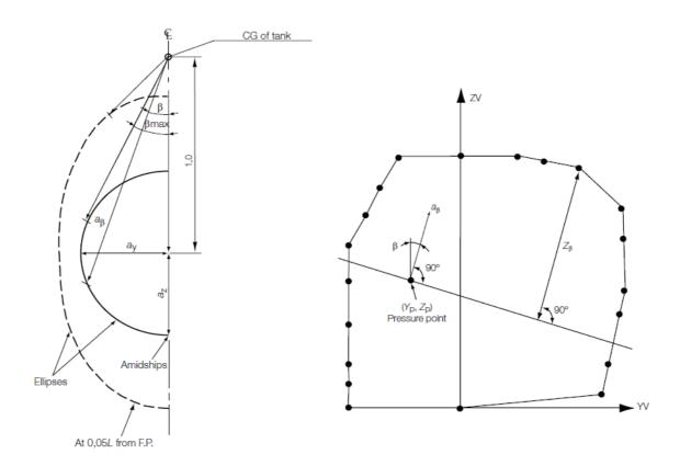
$a_{\beta}=$  resulting acceleration (static and dynamic) in arbitrary direction  $\beta$   $a_{y}=$  transverse component of acceleration  $a_{Z}=$  vertical component of acceleration
