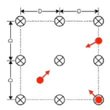
For this system, outer nozzles can be located either at the edge of the protected area or outside of the protected area.
