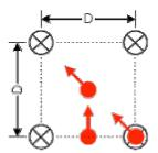
For this system, outer nozzles can be located either at the edge of the protected area or outside of the protected area.
