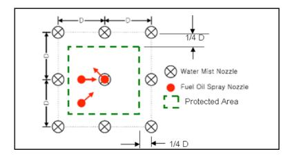
For this system, the outer nozzles should be installed outside of the protected area a distance of at least 1/4 of the maximum nozzle spacing.
