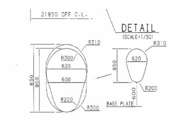
3. If a vertical opening is at a height of more than 600 mm steps and handgrips are to be provided. In such arrangements it is to be demonstrated that an injured person can be easily evacuated.
