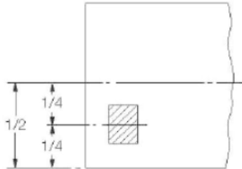
Fig. 1 The location of the test sample
