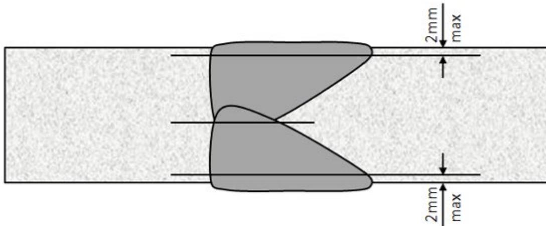
Fig. A 1 Examples of hardness test with rows of indentations in butt welds
